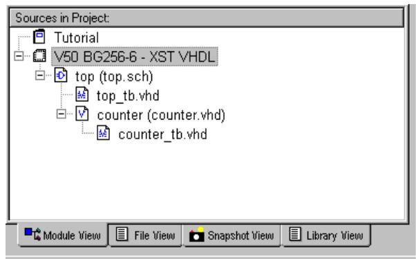
**Figure 4-24 Test Bench File in Source Window**
