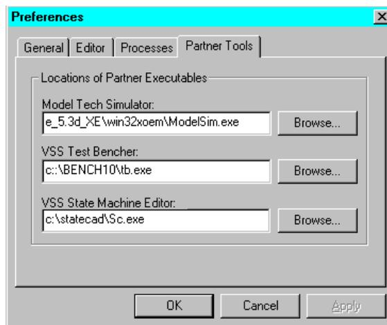
2. Enter the full path name to each of your tools or browse to the location of the desired executable (that is, ModelSim.exe for the Modeltec simulator, tb.exe for the VSS Test Bencher, and Sc.exe for the VSS State Machine Editor).
