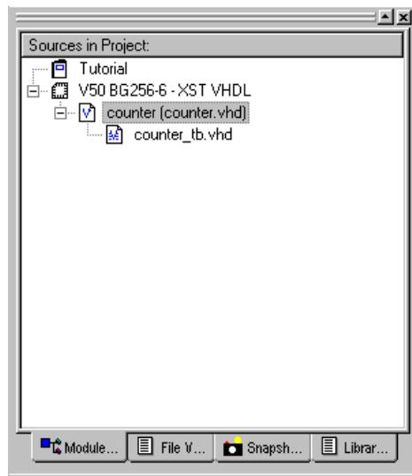
Figure 4-9 Test Bench File in Source Window
