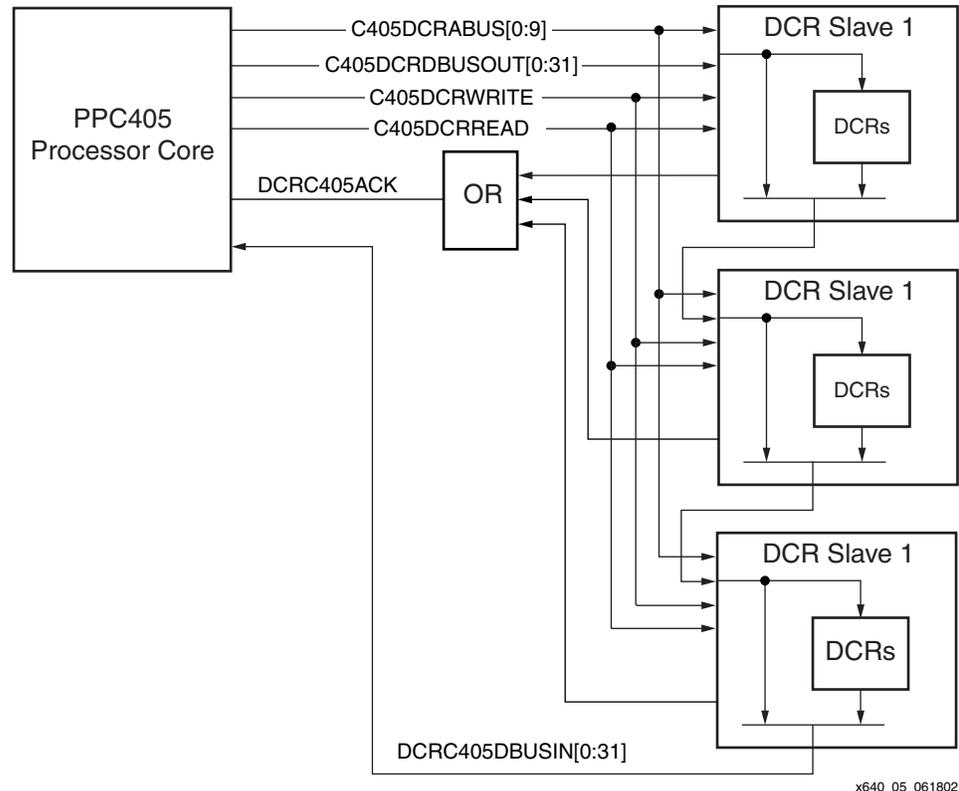
Figure 5: Example CPU DCR Bus
