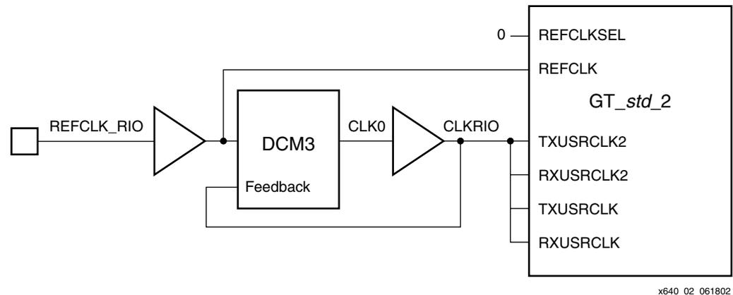
Figure 2: RocketIO DCM Configuration
