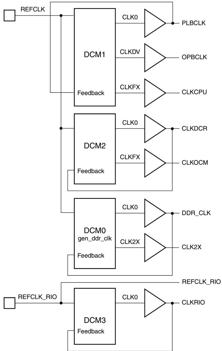
Figure 4: Clocking Structure with Four DCMs
