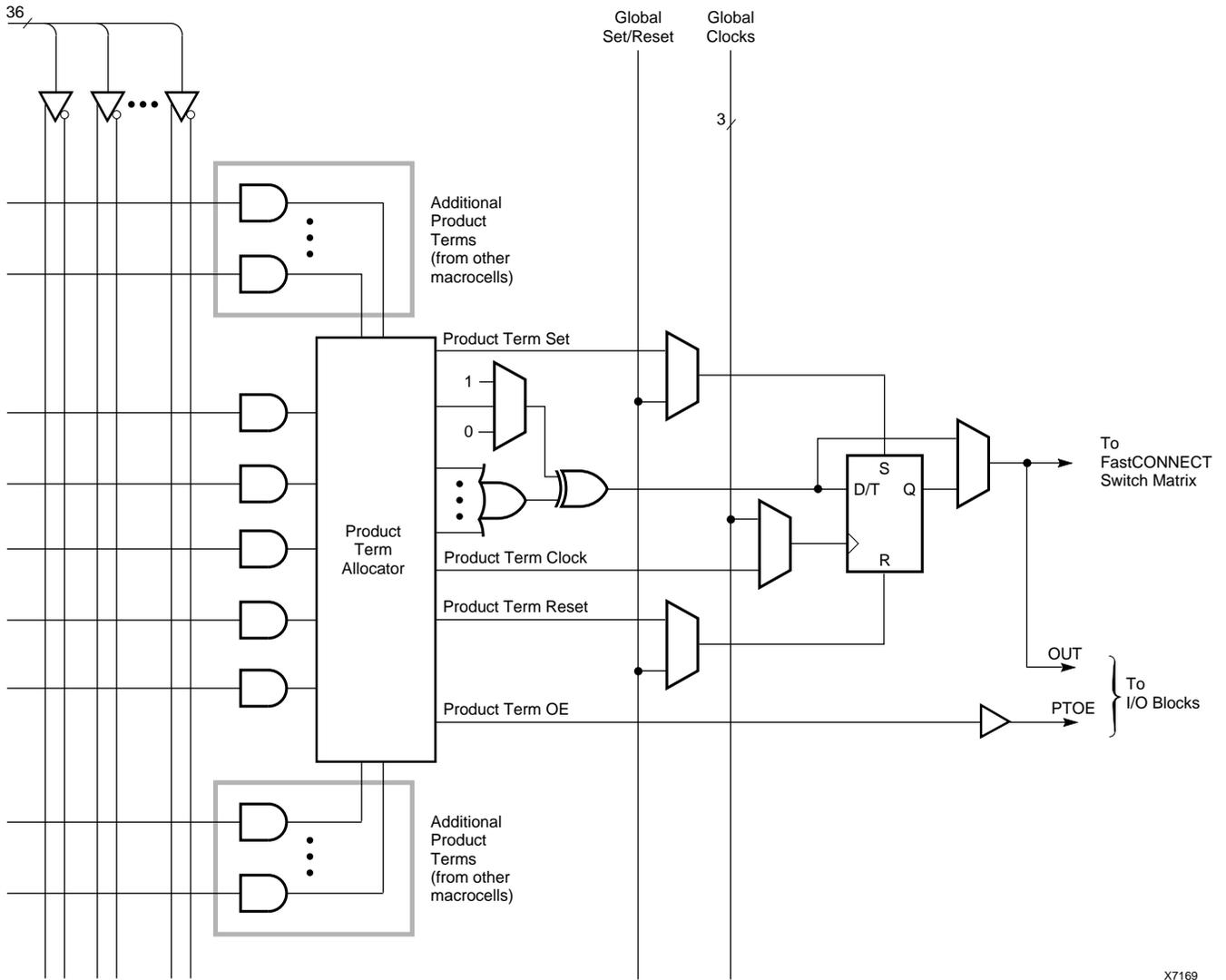
Figure 3: XC9500 Macrocell Within Function Block
