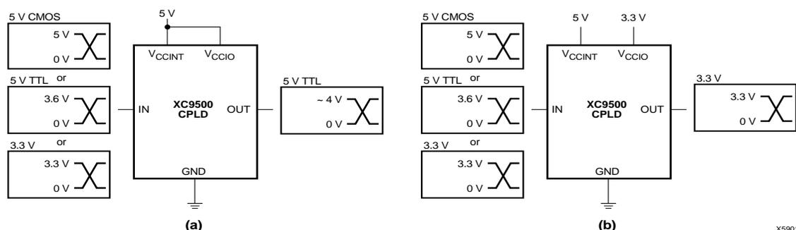
Figure 12: XC9500 Devices in (a) 5 V Systems and (b) Mixed 3.3 V/5 V Systems
