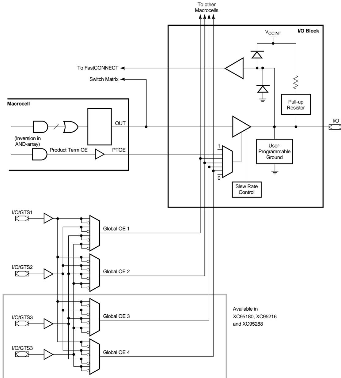
Figure 10: I/O Block and Output Enable Capability
