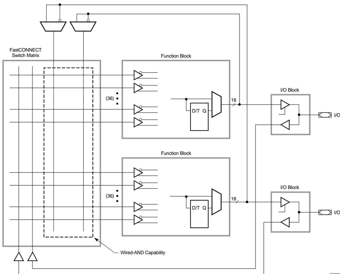
Figure 9: FastCONNECT Switch Matrix
