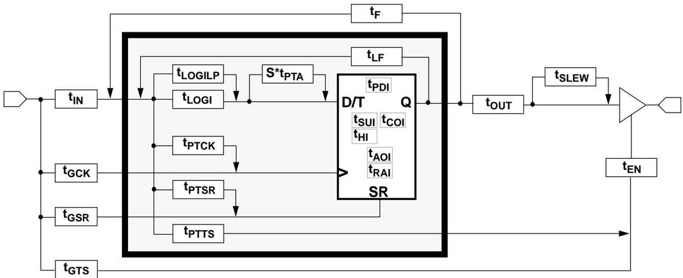
Figure 15: Detailed Timing Model
