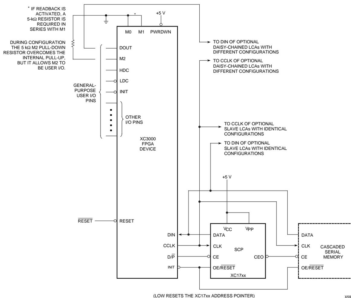
Figure 23: Master Serial Mode Circuit Diagram
