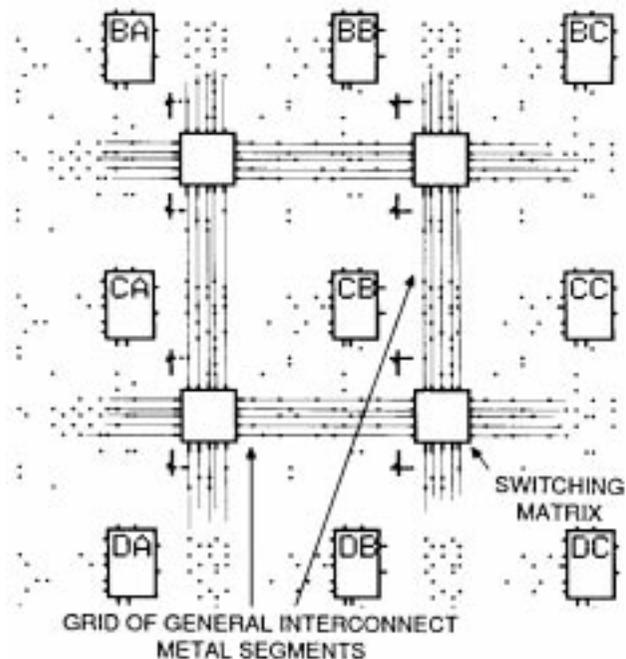
**Figure 10: FPGA General-Purpose Interconnect.**
