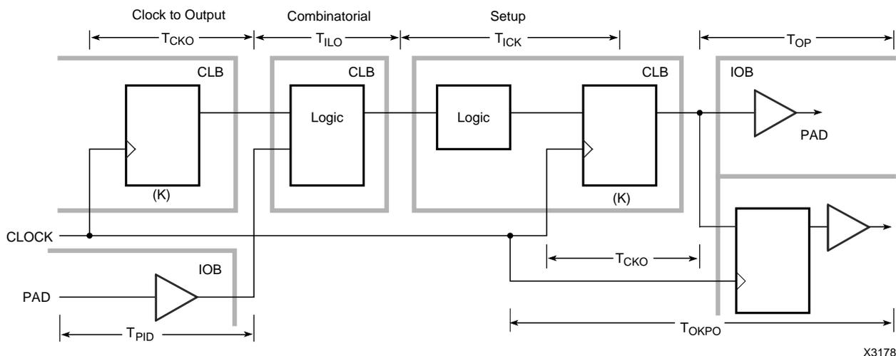
**Figure 31: Primary Block Speed Factors.** Actual timing is a function of various block factors combined with routing factors. Overall performance can be evaluated with the XDelay timing calculator or by an optional simulation.
