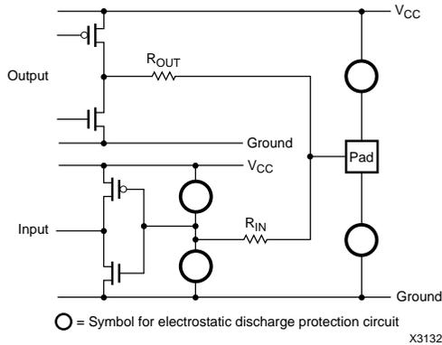
**Figure 3: Input/Output Protection Circuitry**
