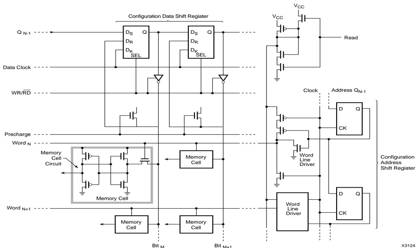
**Figure 2: Configuration Memory Cell**
