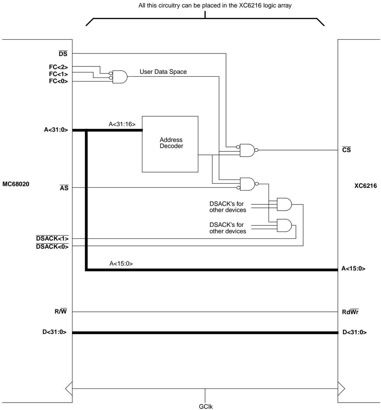
Figure 3. Example Circuit
