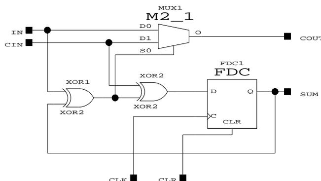
Figure 21. Accumulator Schematic
