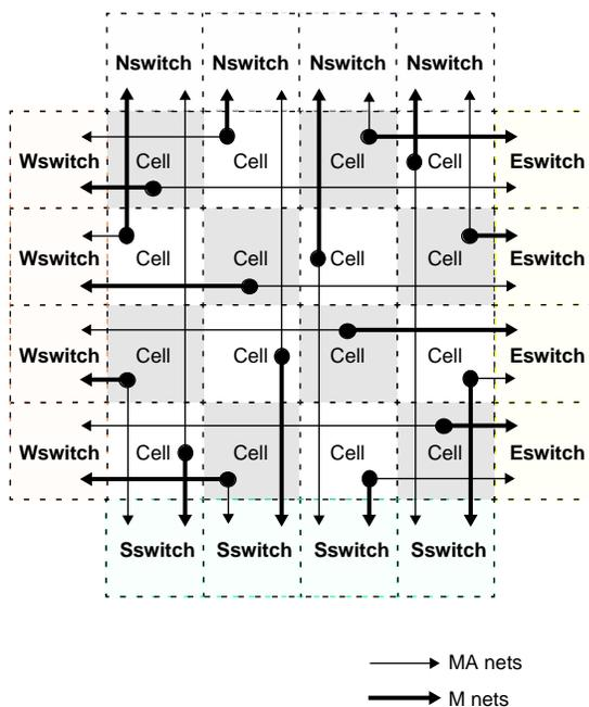
Figure 8. Routing Switches at 4x4 Block Boundary
