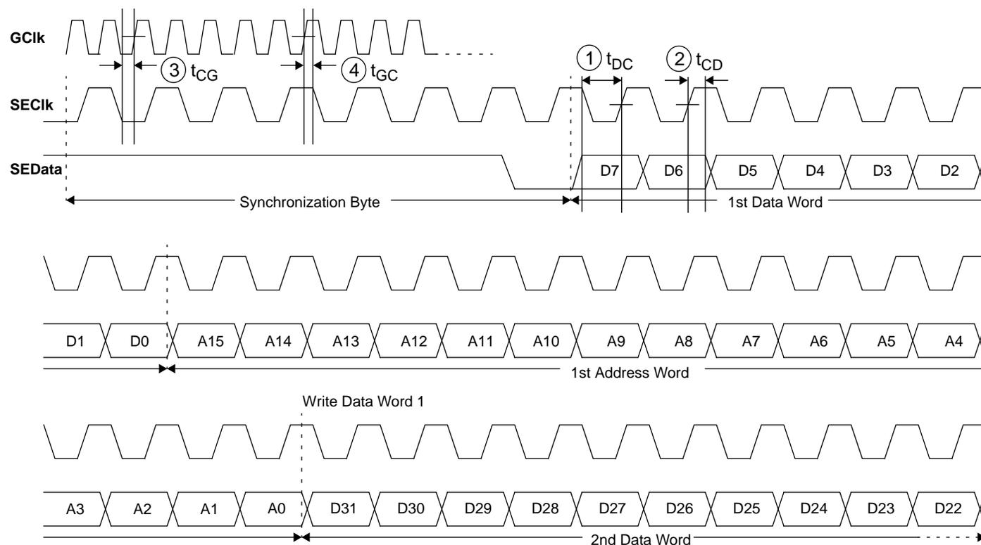
**Figure 28. Serial Configuration Timing**
