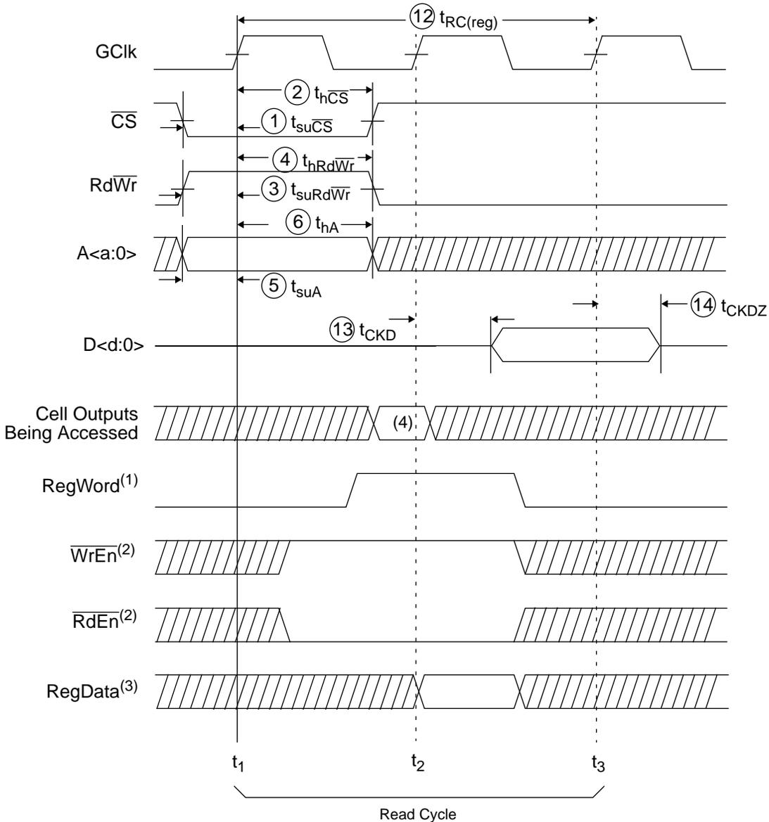
Figure 33. Register Read Cycle
