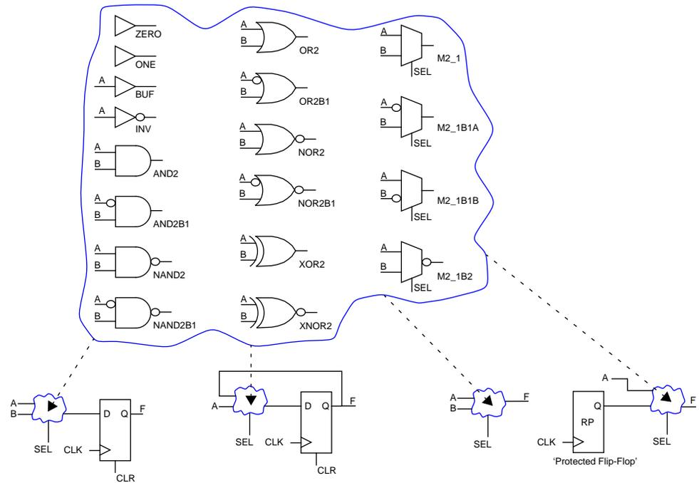
Figure 7. Cell Logic Functions
