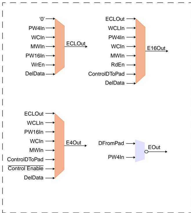
Figure 17. Array Data Sources In West IOBs
