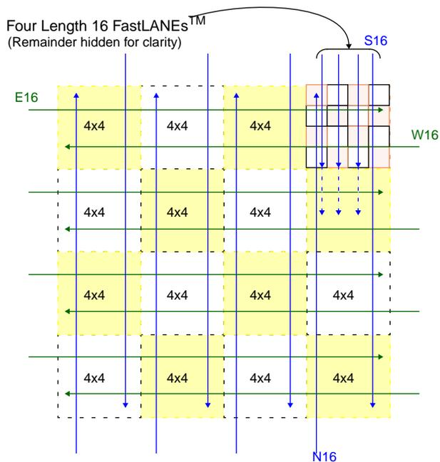
Figure 3. XC6200 16x16 Cell Block
