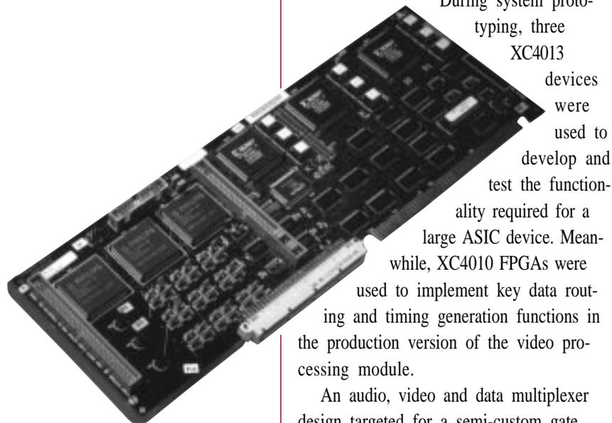
devices were used to develop and test the functionality required for a large ASIC device. Meanwhile, XC4010 FPGAs were used to implement key data routing and timing generation functions in the production version of the video processing module.
