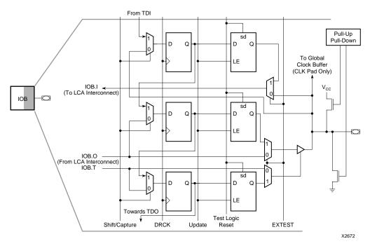
Figure 8-2 XC4000 and XC5200 Boundary Scan Logic in a Typical IOB
