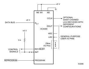
RDY/BUSY pulse. For the Peripheral Synchronous switching characteristics, refer to *The Programmable Logic Data Book*.
