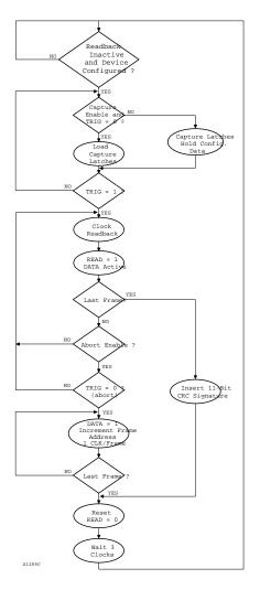
Figure 7-4 Readback State Diagram
