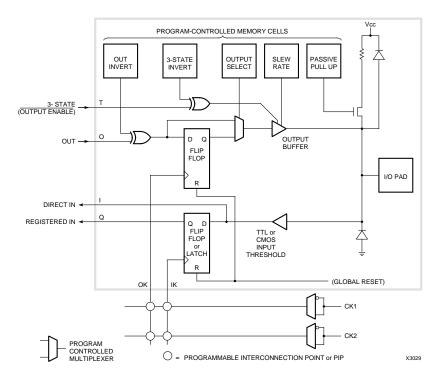
Figure 1-8 XC3000 IOB Structure
