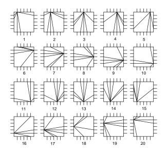
Figure 9-17 Possible Connections in a Switch Matrix
