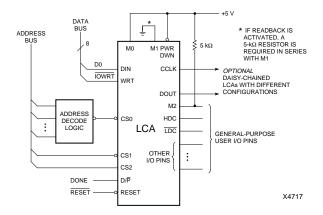
Figure 6-7 Peripheral Mode for XC2000 Devices
