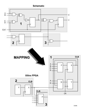
Figure 3-1 Logic Being Mapped into XC3000 CLBs
