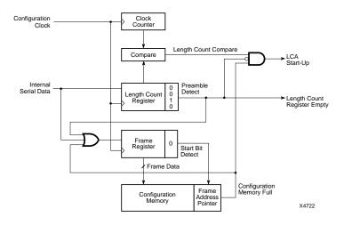
as illustrated by Figure 6-17. The frame register accumulates frames of memory data.
