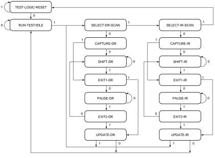
NOTE: The value shown adjacent to each state transition in this figure represents the signal present at TMS at the time of a rising edge at TCK.
