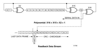
Figure 7-13 Circuit for Generating the CRC-16
