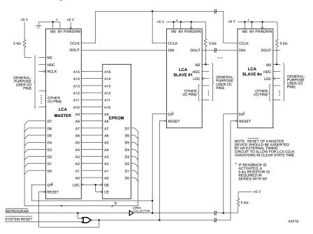
Figure 6-3 Master Parallel Mode for XC2000 Devices
