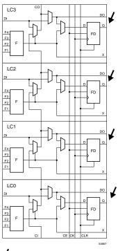
Figure 7-3 illustrates the XC5200 CLB logic configuration.
