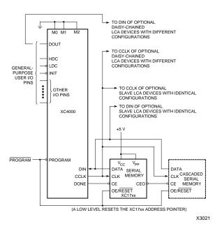
Figure 6-12 illustrates the Master Serial mode for the XC4000 and XC5200 devices.
