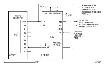
Figure 6-9 Slave Serial Mode for XC2000 Devices
