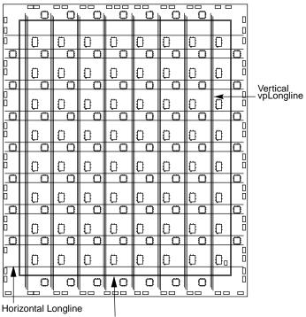
Four Outer Longlines are Connectable Half-Length Lines
