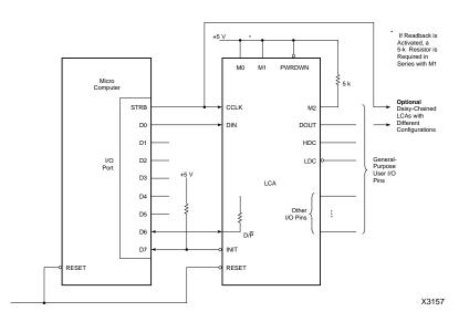
Figure 6-10 Slave Serial Mode for XC3000/XC3100 Devices
