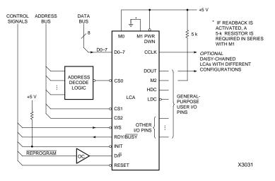
Figure 6-8 shows the parallel data Peripheral mode connections of the XC3000 devices.
