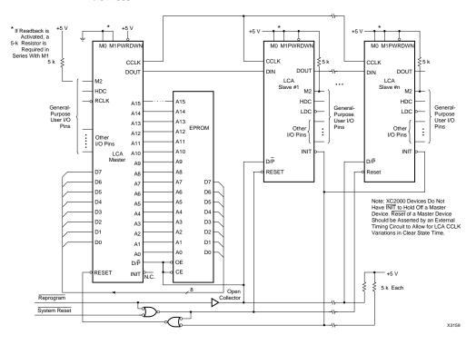
Figure 6-4 illustrates the Master Parallel mode for XC3000/XC3100 devices.
