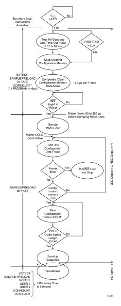
Figure 6-20 State Diagram for XC4000 and XC5200 Configuration
