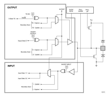
Figure 1-7 XC4000H IOB Structure
