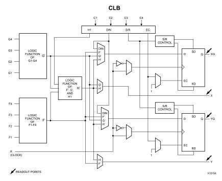
Figure 7-2 illustrates the XC4000 CLB logic configuration.
