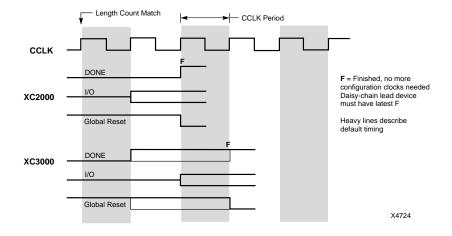
Figure 6-19 Start-up Timing for XC2000/XC3000 Devices
