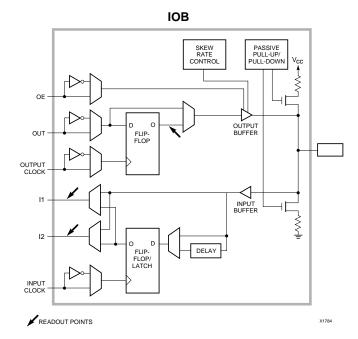
Figure 7-1 XC4000 IOB Logic Configuration
