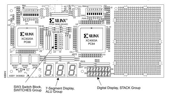
Figure 10-14 FPGA Demonstration Board Components
