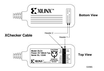
Figure 4-2 XChecker Cable Pins
