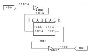
Figure 10-2 Readback Symbol Connections
