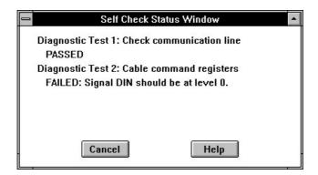
Figure 8-30 Failed Self-Check Test
