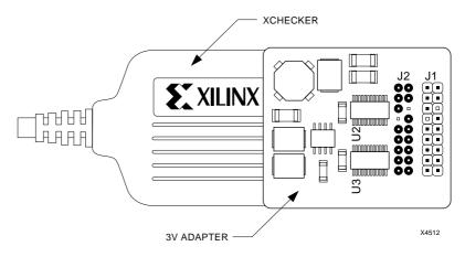
Figure A-2 XChecker 3-Volt Adapter
