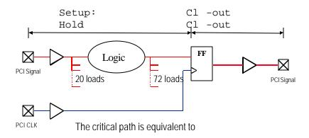
Xilinx supports this path in its Virtex FPGA family, and it is implemented and guaranteed in Xilinx Real 64/66 PCI core design. Furthermore, Xilinx guarantees the 0 ns hold-time and both the 6 ns max clock-to-out and 2 ns min clock-to-out.
