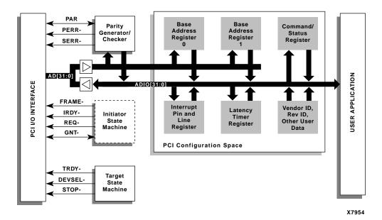
Figure 1: LogiCORE PCI32 SpartanXL Interface Block Diagram (one BAR only in XCS20XL)
