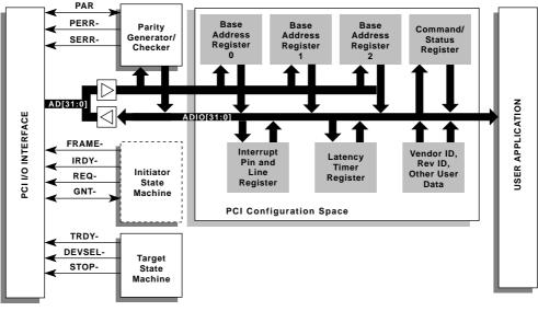
Figure 1: LogiCORE PCI32 Interface Block Diagram
