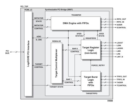
Figure 1: Block Diagram of Synthesizable Bridge Design for PCI64 LogiCORE Interface, SB07
