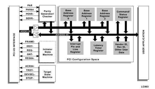
Figure 1: LogiCORE<sup>™</sup> PCI64 Interface Block Diagram
