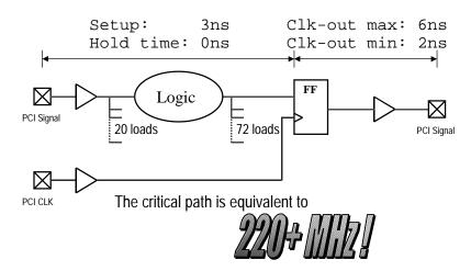
Figure 1: The critical path for 0 wait-state PCI64/66
