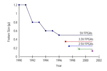
Figure 3: Accelerated FPGA process migration enabled by a structural repetitive architecture
