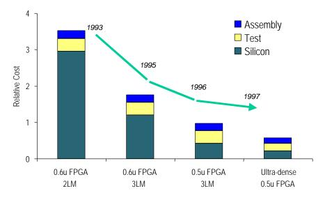
Figure 2: Silicon cost becomes a smaller component of total cost with denser processes
