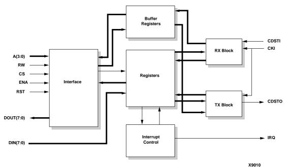
Figure 1: HDLC Controller Block Diagram
