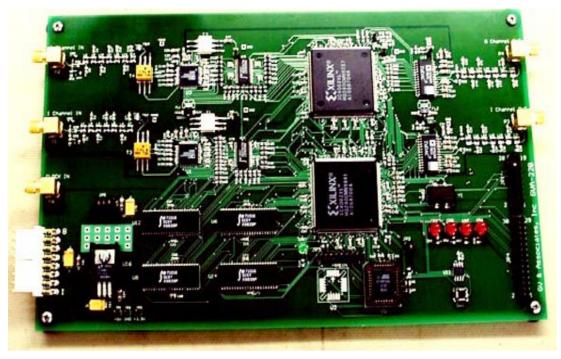
Figure 1: GVA-220 DSP Hardware Accelerator
