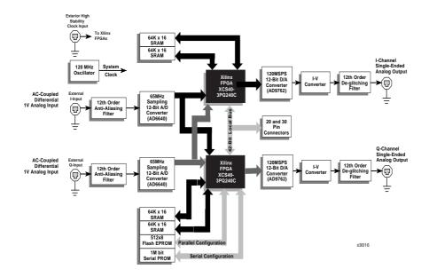
Figure 2: GVA-220 Spartan FPGA Block Diagram
