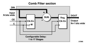
Figure 1. Block Symbol and Schematic Diagram
