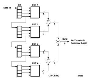
Figure 3. Combining 4-Input Sections
