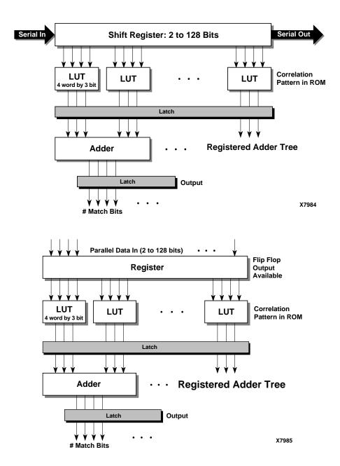
Figure 2. CORE Generator Implementation for Serial Data (top) and Parallel Data (bottom)
