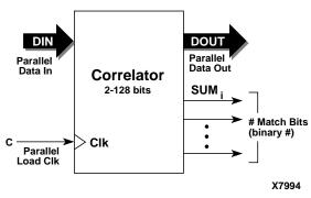
Figure 5. Core Schematic Symbol - Parallel Data In
