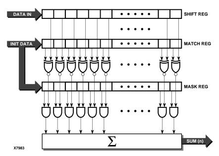
Figure 1. Serial In Correlator Block Diagram
