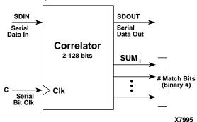
Figure 4. Core Schematic Symbol – Serial Data In Table 2. Core Signal Pinout – Serial Data In
