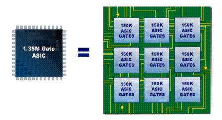
Designers now struggle with the problem of breaking up their ASIC into multiple FPGAs for prototyping. This is a tedious task often performed by the most experienced designers. Today, partitioning and synthesis are two separate steps. The user must partition logic blocks into FPGA size blocks, then synthesize each block into FPGA specific technology libraries. If the partitions do not fit into the desired FPGAs, the
