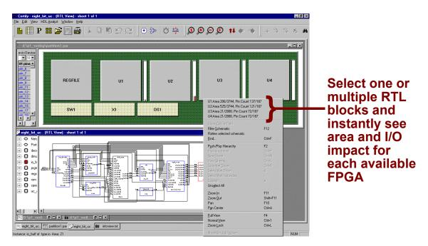
The Certify tool's ability to report logical and physical connectivity allows it to guide the partitioning process over a variety of emulation platforms e.g. re-configurable platforms, pre-defined boards or Certify-created boards.
