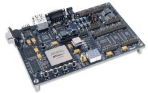
The Nios Development Kit, Stratix Edition featuring the EP1S25 device.
